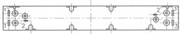
P.C.B. MOUNTING DETAIL
